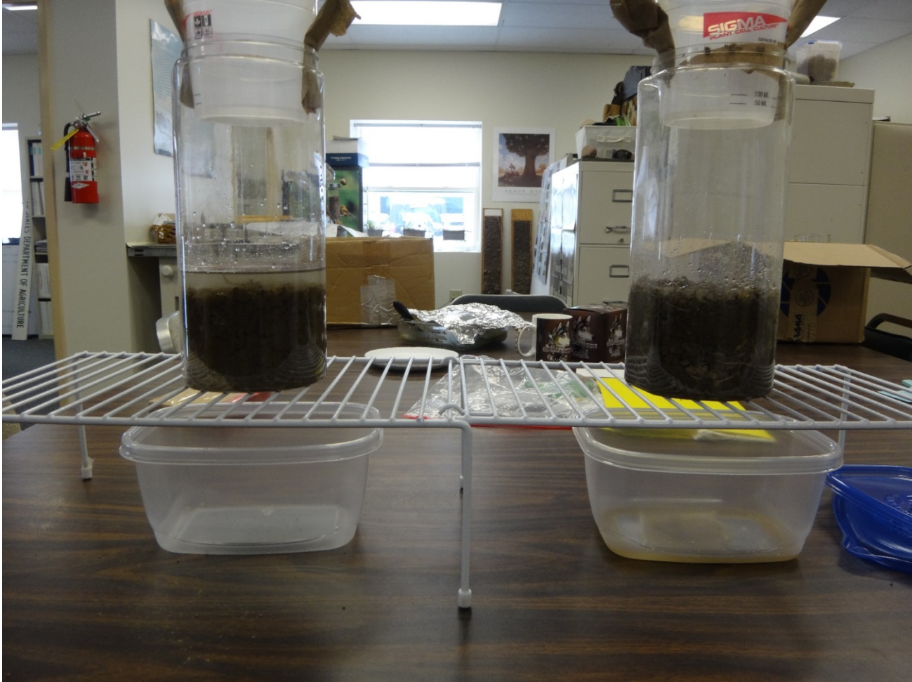
Fig. 2. Columnar infiltration demonstration, with the long term conventional tillage system on the left resulting in less stable aggregates which seal the soil surface and reduce infiltration and permeability, resulting in ponding, compared to soil from long term sod which allows more infiltration and permeability.
