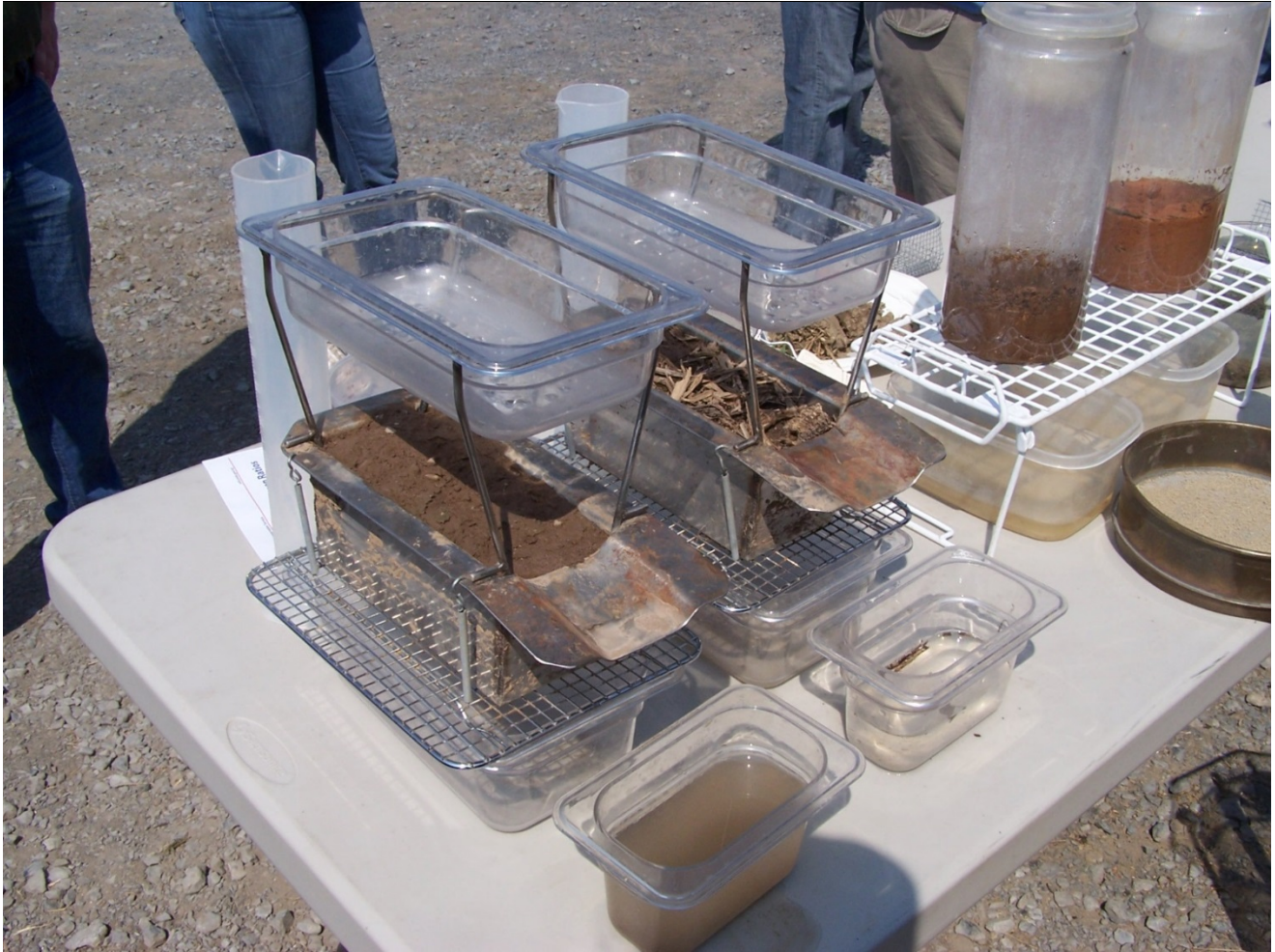
Fig 3. The table top rainfall simulation demonstration, with the long term conventional tillage system on the left resulting in poor infiltration and more runoff carrying sediment. The no-till soil on the right results in more infiltration, percolation, water storage and cleaner runoff.
